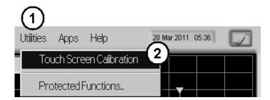
2 Touch the center of the X with your finger or a stylus. Several X will appear on different positions of the display screen. Touch them precisely as the first one. When the display is calibrated, the touch screen configuration utility closes.
